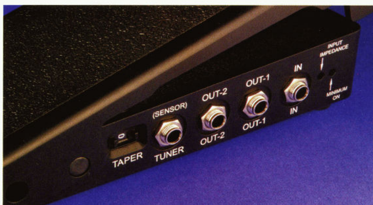
One input, two identical outputs, a socket for a tuner or remote controller, a digital preset selector and mini-pots for impedance and 'minimum on' settings
